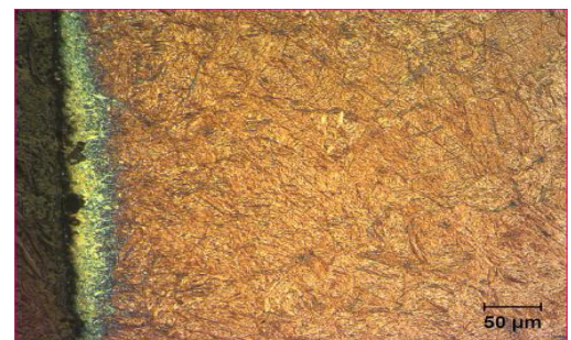
Fig. 11. Sample treated at 930 °C for 3 hours ×200
